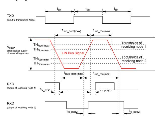
Figure 6.5: Definition of bus timing parameters
