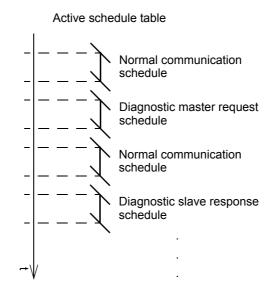
Figure 5.7: Normal diagnostic communication mode
