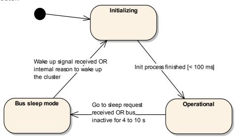
Figure 2.15: Slave node communication state diagram
