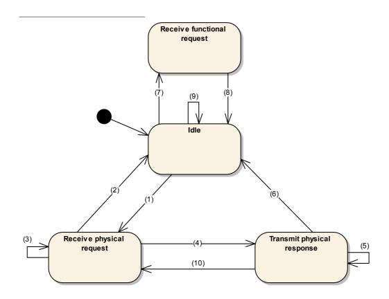
Figure 5.12: Slave node transmission handler
