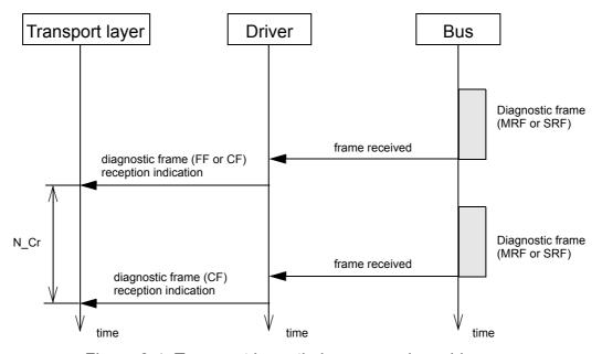
Figure 3.4: Transport layer timing on receiver side
