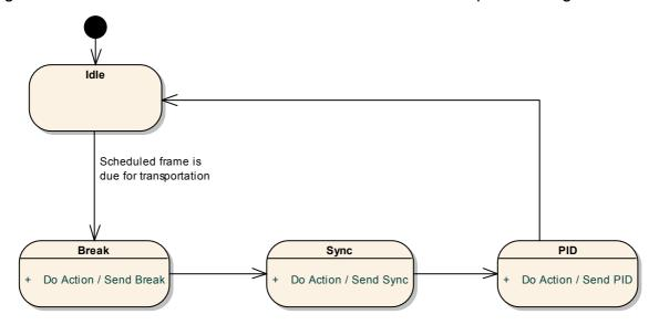
Figure 2.13: Complete state machine for the master task.
