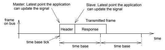
Figure 2.2: Timing of signal transmission
