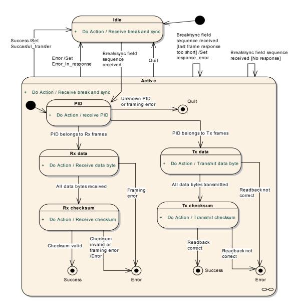
Figure 2.14: Frame processor state machine.
