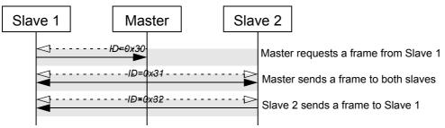
Figure 2.9: Three unconditional frame transfers.
