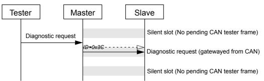
Figure 5.1: Gatewaying of CAN messages to LIN.
