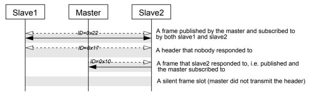
Figure 2.19: Frame sequence example.
