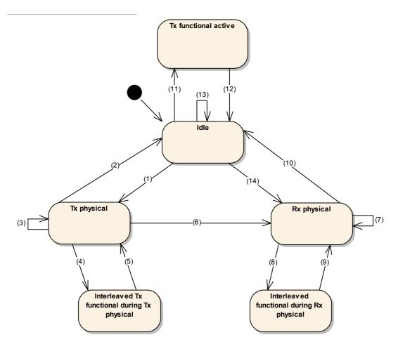
Figure 5.11: Master node transmission handler
