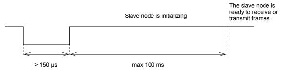
Figure 2.16: Wake up signal reception in slave nodes
