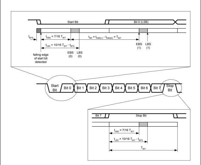
Figure 6.2: Bit Sample Timing
