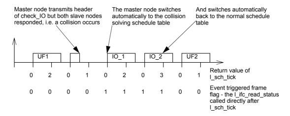
Figure 7.1: Event triggered frame collision solving example
