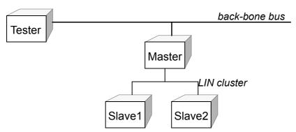
Figure 3.1: Typical system setup for a LIN cluster using the transport layer.
