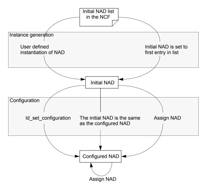
Figure 4.2: NAD instantiation and configuration process
