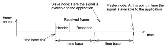
Figure 2.1: Timing of signal reception
