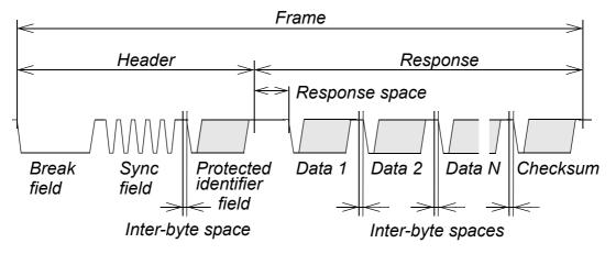
Figure 2.3: The structure of a frame.
