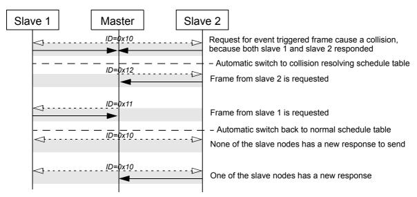
Figure 2.10: Event-triggered frame example.
