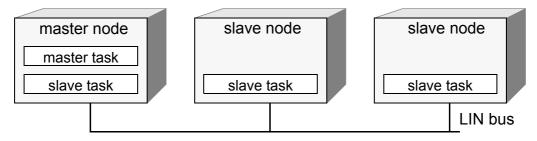
The master task decides when and which frame shall be transferred on the bus. The slave tasks provide the data transported by each frame.
