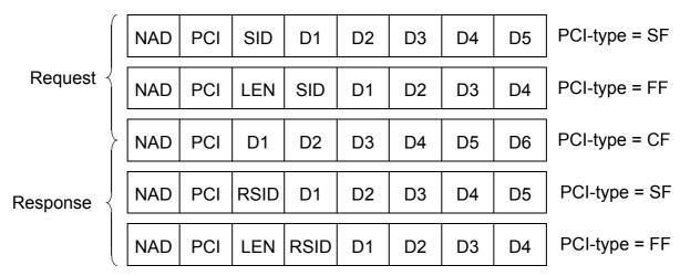
Figure 3.2: PDUs supported by the LIN transport layer.
