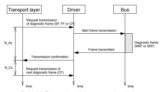
Figure 3.3: Transport layer timing on transmitter side
